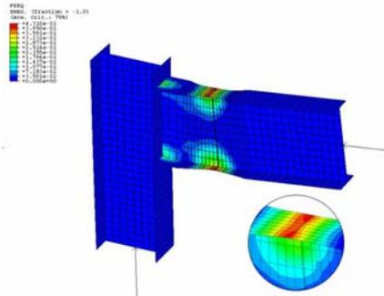
Figure 15. Cumulative plastic strain at end of earthquake
