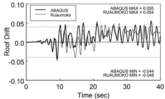
Figure 14. Roof drift under 3.366xrecord
