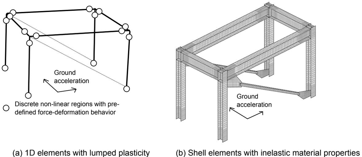
Figure 2. Models used for dynamic analysis
