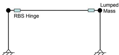
Figure 7. 1D Model with Plastic Hinges
