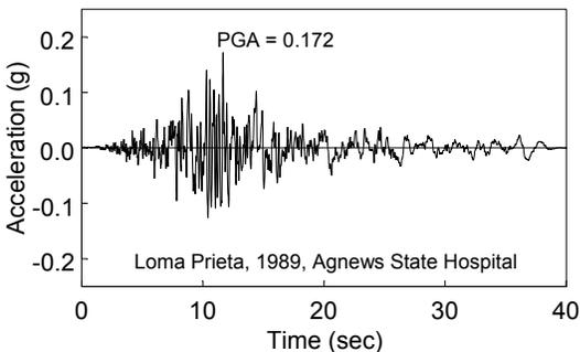
Figure 9. Earthquake record used for analyses
