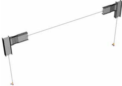
Figure 11. ABAQUS model with refined mesh in connection regions
