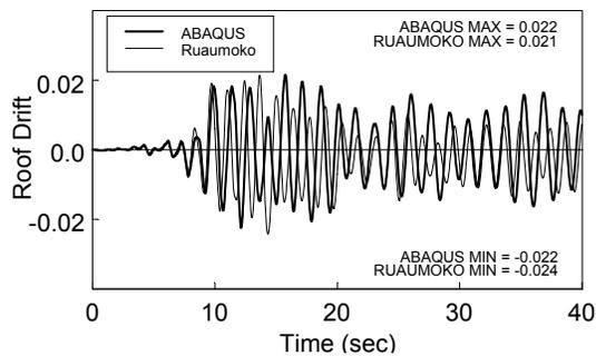
Figure 13. Roof drift under 1xrecord
