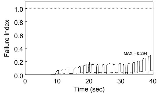
Figure 16. Failure index at RBS connection
