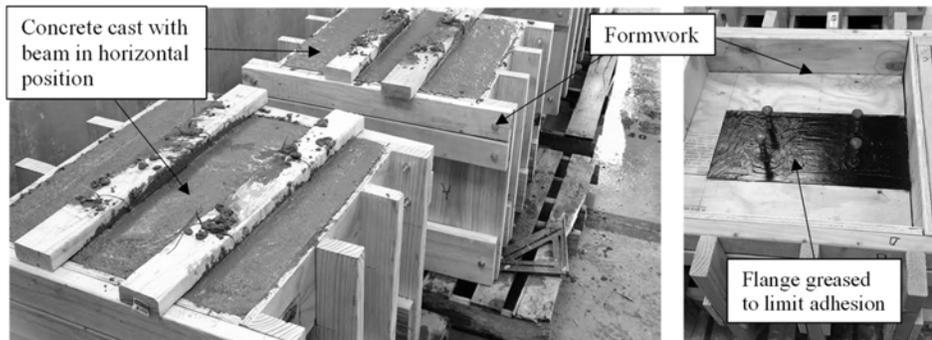
Figure 4. Casting of concrete slabs on double sided push-out specimens
