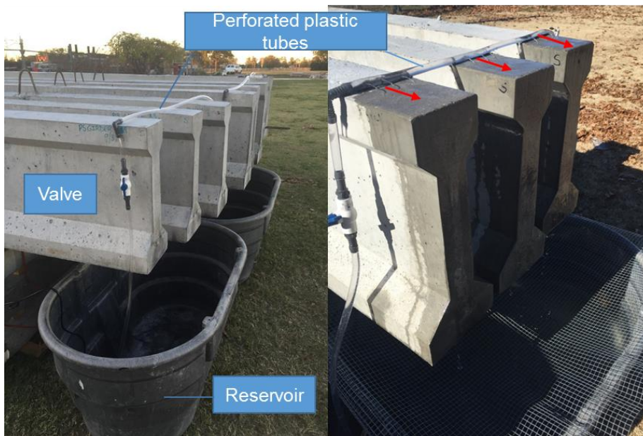
Figure 1. Completed girders placed in corrosion accelerant setup (red arrows indicate the direction of flow from the perforated tubes)
