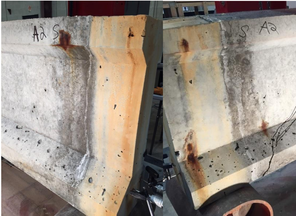
Figure 2. Example of a corroded beam end after the accelerated corrosion process.
