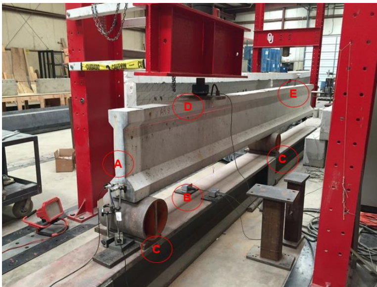
Figure 3. Typical shear test setup looking towards the north – (A) LVDT 1 & 2, (B) wire pots 1 (west) & 2 (east), (C) supports at 9 ft center-to-center, (D) single load point with load cell at 41 in. from end of beam, and (E) 8 ft - 8 in. overhang of the beam
